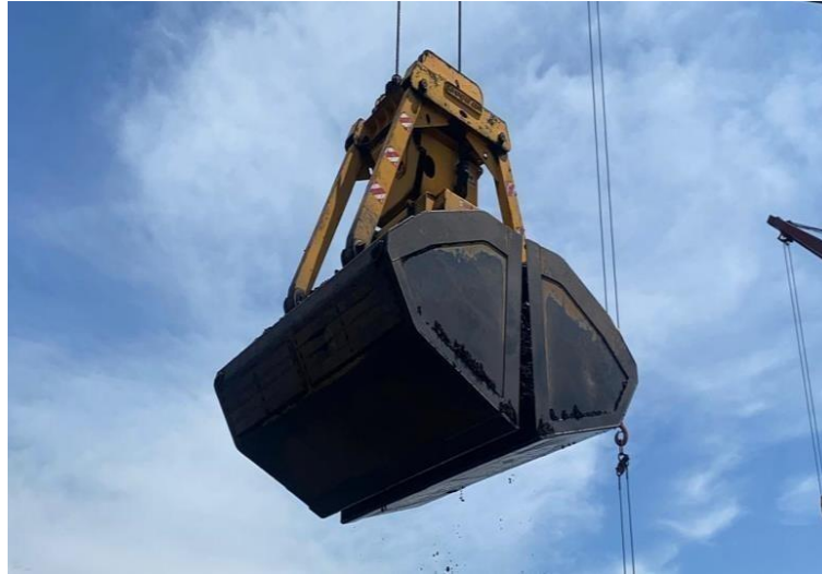
Figure 7. Grab not fully closed
