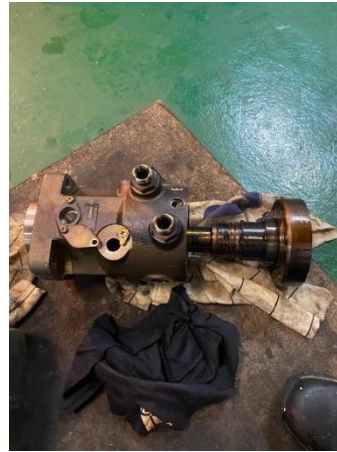
Figure 4. Fuel oil pump
