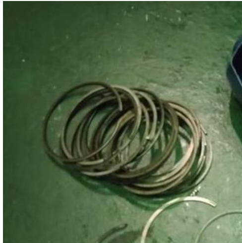
Figure 1. Used Piston Rings Removed from the Auxiliary Engine
