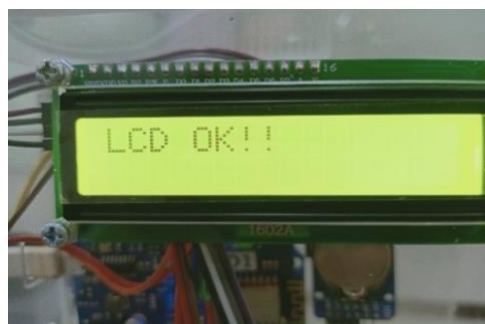
Figure 6 I2C Test Results
