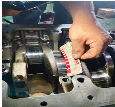
Figure 1. Oil clearance measurement
