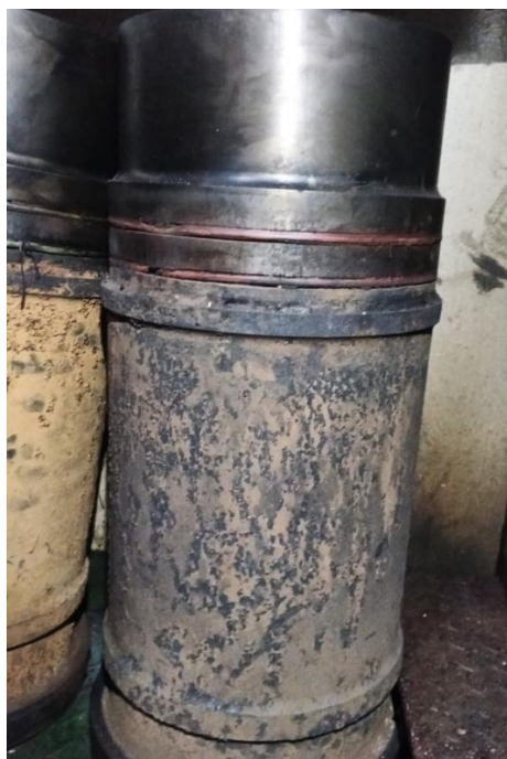
Figure 4 Oring Cylinder liner replacement
