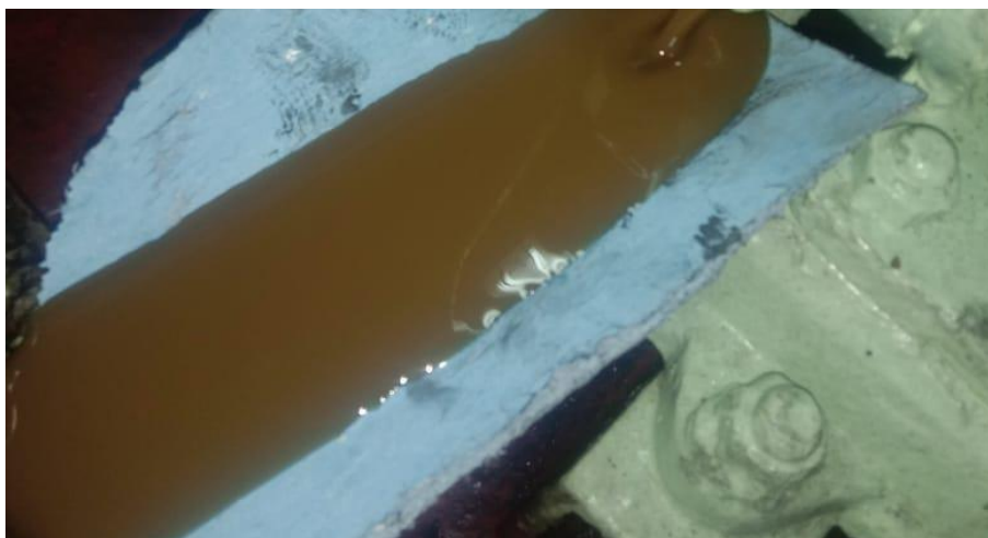
Figure 2 Lubricating oil mixed with water
