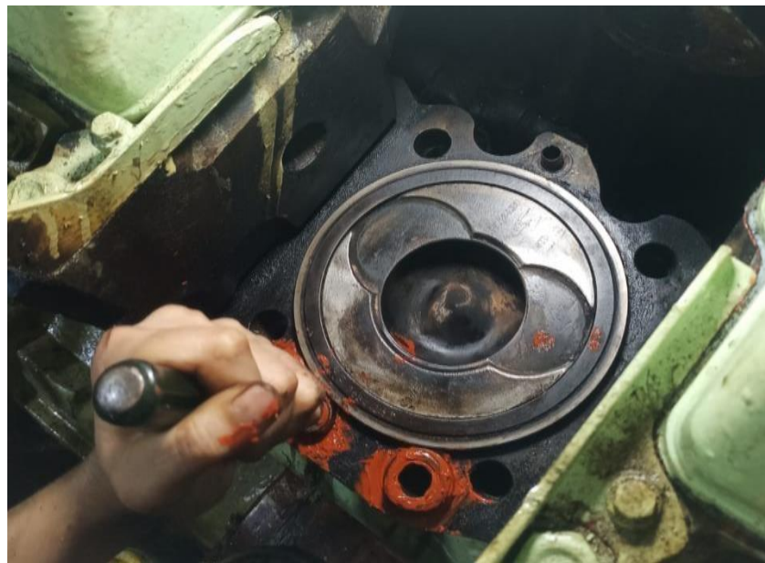
Figure 3 Suspected Damage to O ring Cylinder Join in Cylinder Head
