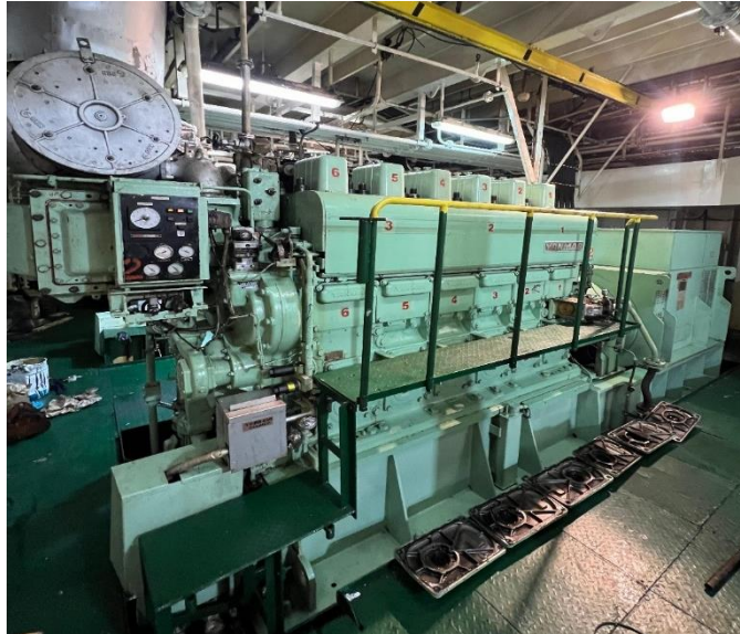
Gambar 1 Diesel Generator Yanmar 6-CYL. / EY26L
